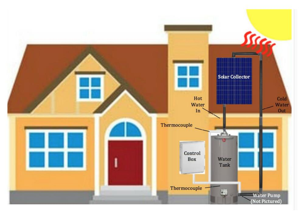
The control box utilizes an arduino and thermocouples connected to the hot water tank to determine whether water heating is necessary. If the temperature is too low then water is pumped through the solar collector to be heated and then stored in the hot water tank.
